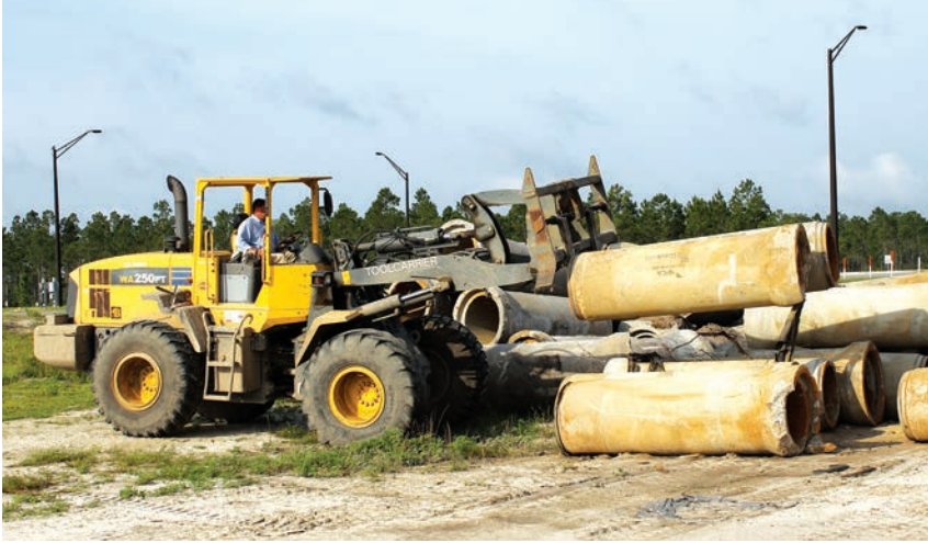
Gulf Coast Utility Contractors has several Komatsu wheel loaders in its equipment fleet, including this WA250 parallel tool carrier.
